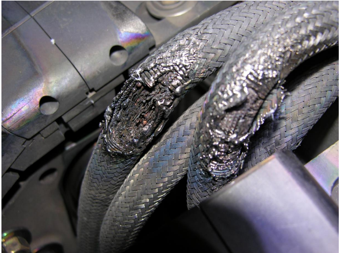
Close-up of damaged XTOMO signal cables
